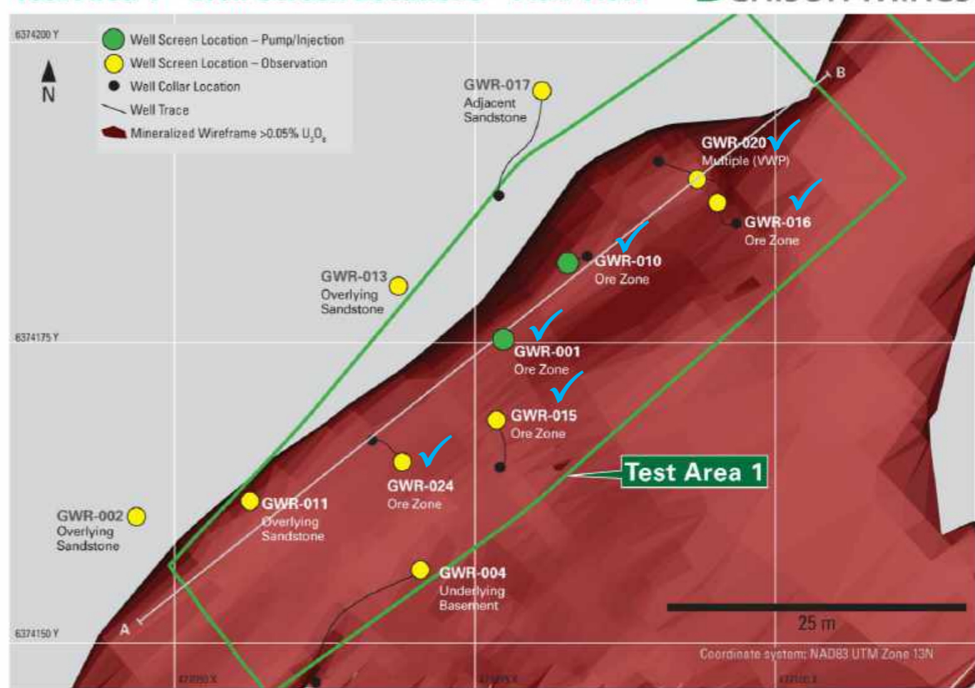
Test Area 1 – Well Screen Locations – Long Section
